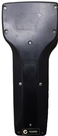
Figure 3 Removing the Back Panel of the Pro Cab or Power Cab
