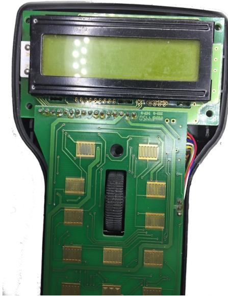
Figure 11 The main circuit board replaced
