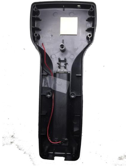
Figure 7 Route the leads carefully to the left of the battery compartment and tape them down.
