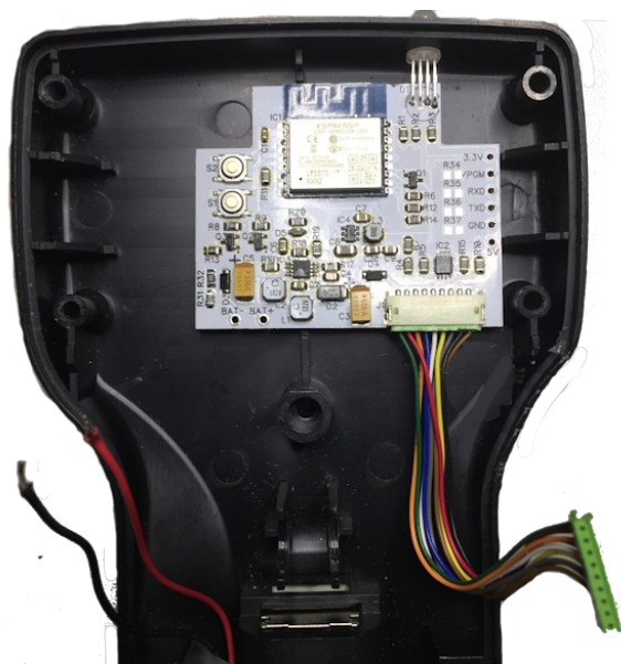
Figure 8 Connect the 9-way cable to the WNI-32 module
