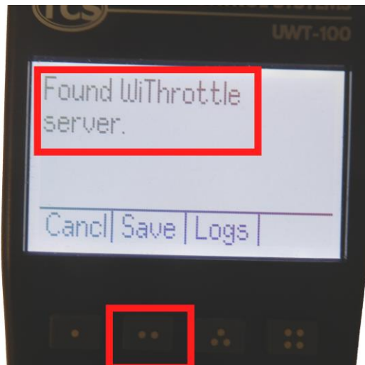
Figure 20 The WFD-60 WiThrottle server has been found. Now save it!
