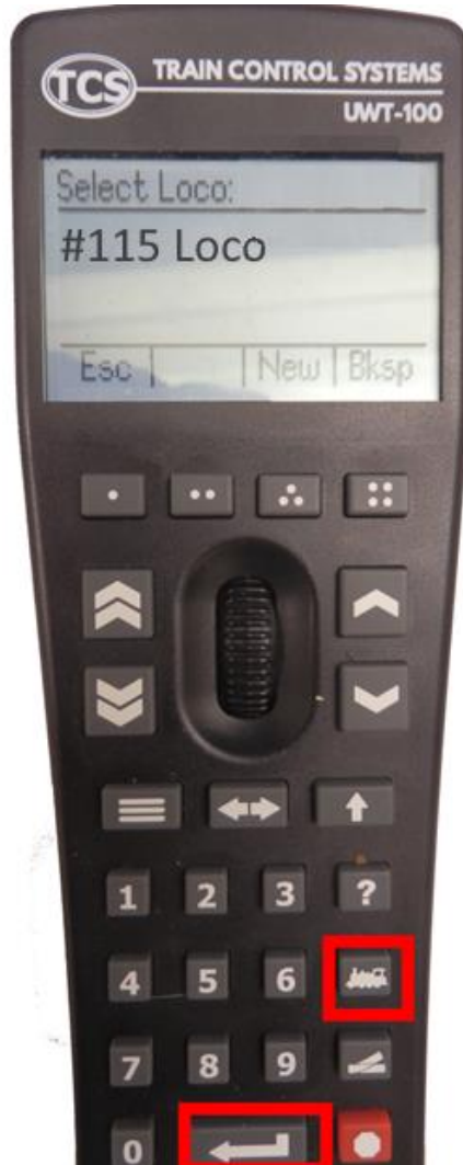
Figure 21 Select a Locomotive from the Roster – in this case the only one.
