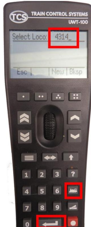
Figure 26 Select a locomotive with a known DCC address
