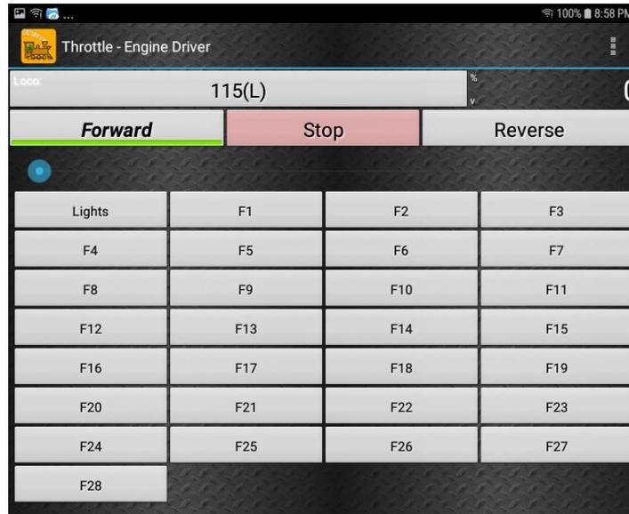
Figure 23 The Throttle screen of Engine Driver with a locomotive selected to drive
