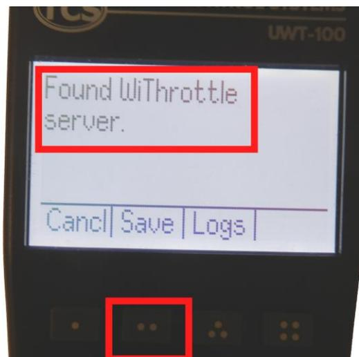
Figure 28 The WFD-28 WiThrottle server has been found. Now save it!
