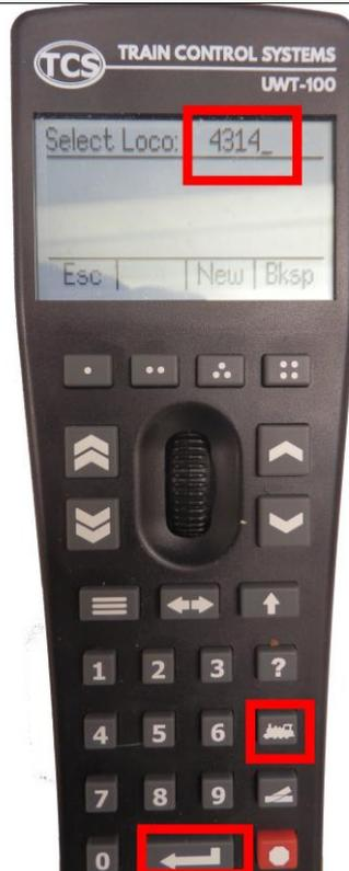
Figure 29 Select a locomotive with a known DCC address
