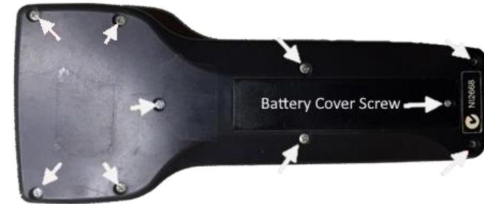
Figure 14 The nine screws holding the back on a Pro Cab. The tenth, smaller screw secures the battery cover
