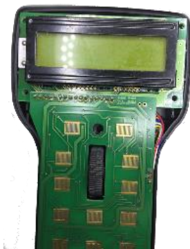
Figure 13 Replace the main PCB in the Pro Cab. Make sure all the wires are free and none are trapped.
