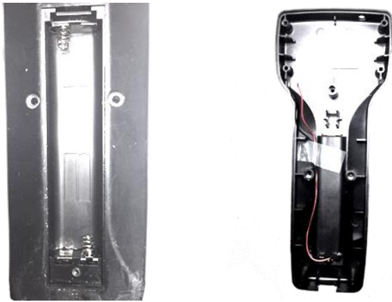
Figure 16 Installing the Battery Connectors and routing the leads
