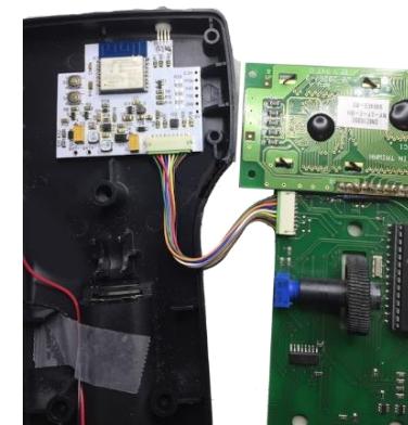
Figure 18 Connect to the main PCB of the Pro Cab
