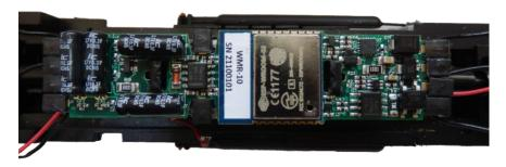
(1) Figure 3 WMR-10 Installed in a locomotive. Here the wires have been attached using the original plastic clips.
