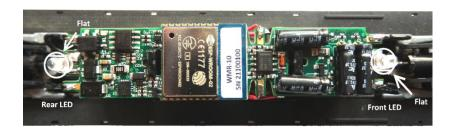
Figure 2 WMR-10 Installed in a locomotive. Here the wires and the LEDs have been soldered to the tabs on the module.
