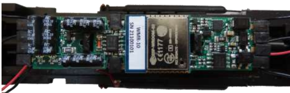
Figure 3 WMR-10 Installed in a locomotive. Here the wires have been attached using the original plastic clips.
