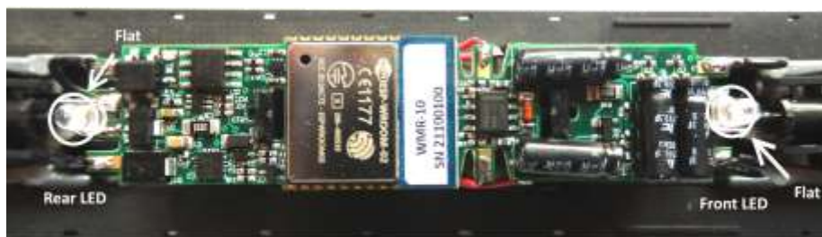
Figure 2 WMR-10 Installed in a locomotive. Here the wires and the LEDs have been soldered to the tabs on the module.
