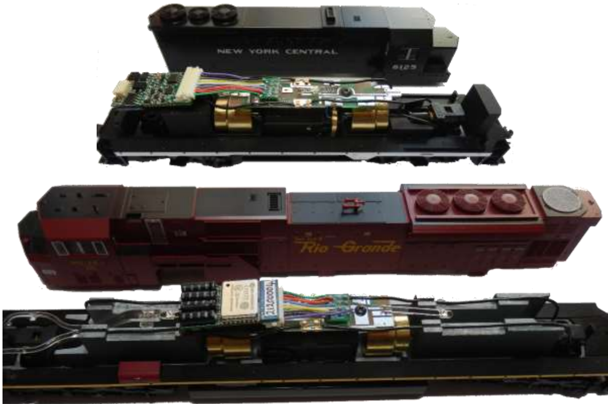
Figure 2 Typical WMH-20 Installations. Always put a piece of electrical tape underneath!
