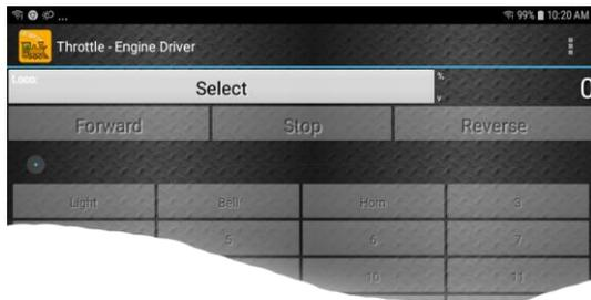
(12) On the Select/Release Loco screen, check the “Roster” option and select the loco that you wish to drive. You cannot select locos by DCC address using the WFD-60.
