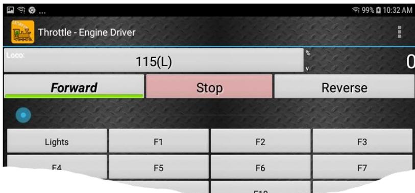
If you have been using an app on your phone to drive trains, via a computer running JMRI, you can now bypass JMRI and connect your phone directly to the WFD-60.
