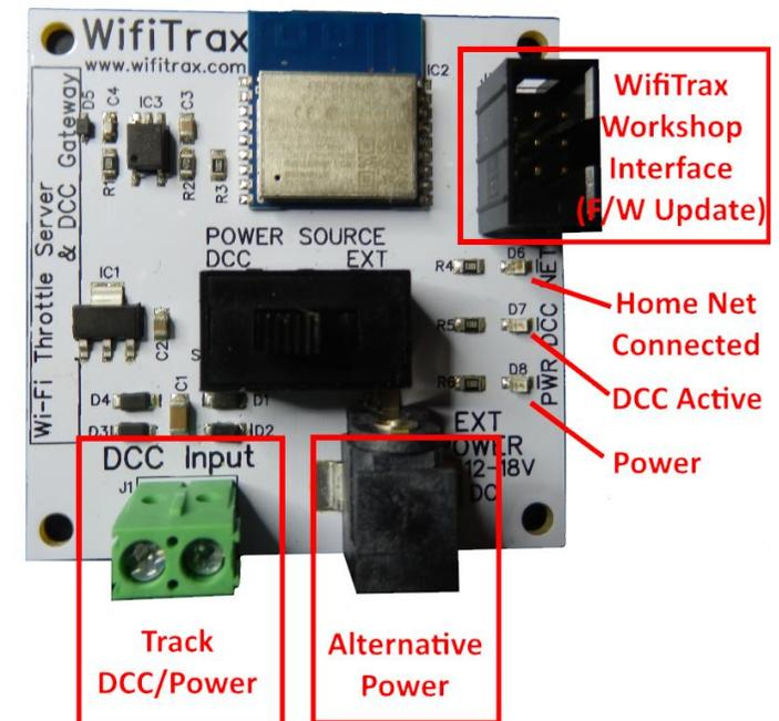
Figure 1. WFD-60 Connections
