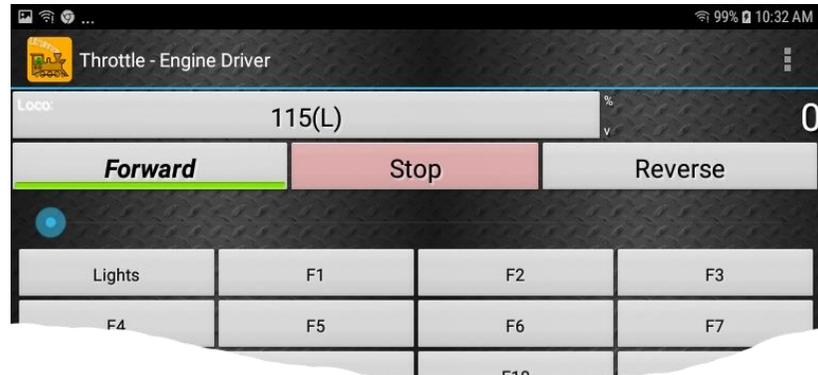
If you have been using an app on your phone to drive trains, via a computer running JMRI, you can now bypass JMRI and connect your phone directly to the WFD-60.
