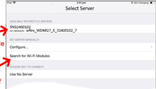
The module's WiThrottle server has been found. Tap to connect.
