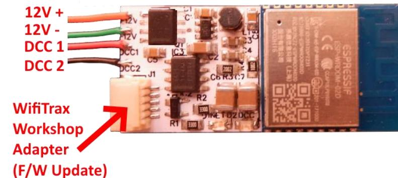
Figure 1. WDMI-32 Connections
