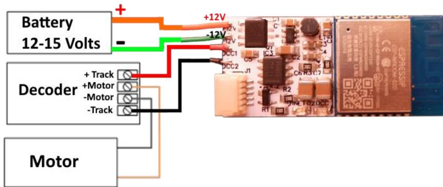
Figure 2. Connections to the WDMI-32
