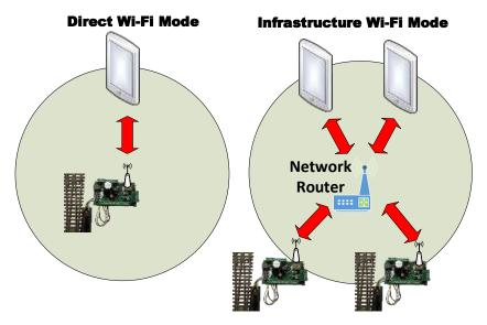
The first thing to understand is that there are two ways of controlling your layout features over Wi-Fi, Direct Mode and Infrastructure Mode.
