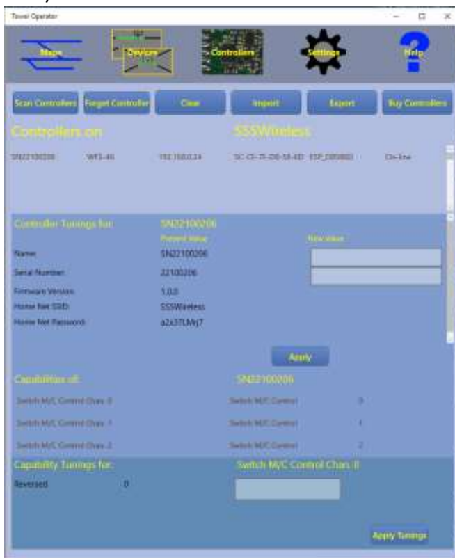
Figure 15. The controller now Appears on the Home Network when that Network is Chosen as the Operating Network
