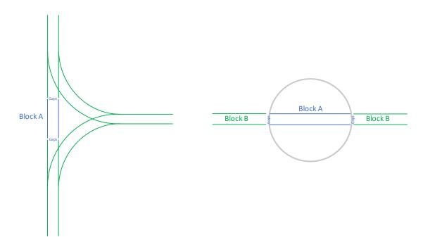
Figure 3 The Wye and Turntable Track Configurations
