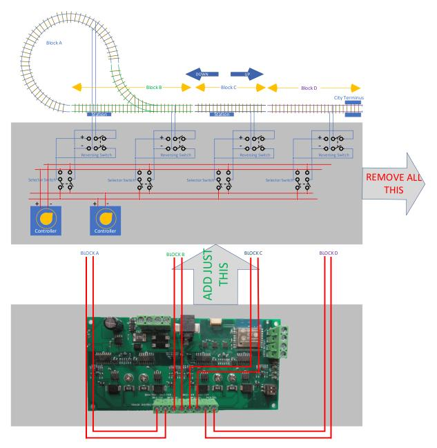
Figure 4 Converting a DC Layout to Wi-Fi DC with one WUFP-40 Module
