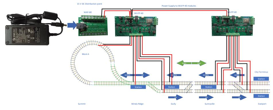
Figure 6 Power Wiring of the Sunny Valley DC Layout
