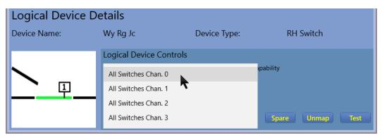
Figure 23 Selecting the Physical Controller Capability for a Logical Device
