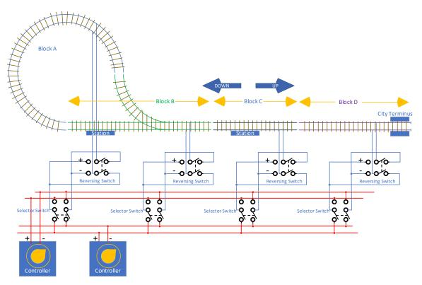
Figure 2 A Part of a Model Railroad with a more Complicated Block System
