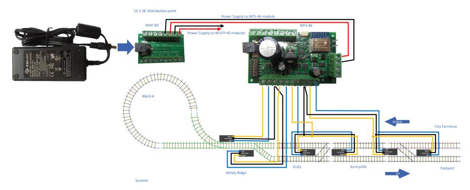
Figure 7 Switch Machine Wiring using the WFS-46
