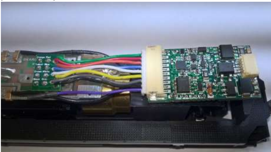
Figure 10 The WMH-20 module and its harness installed in the locomotive.
