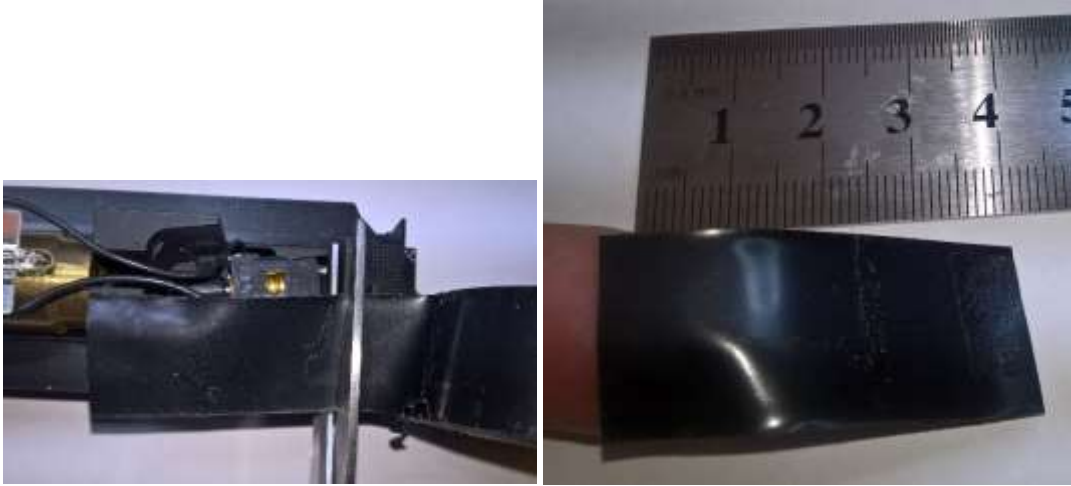
Figure 7 Cut a length of electrical tape, 4 cm should be about right.
