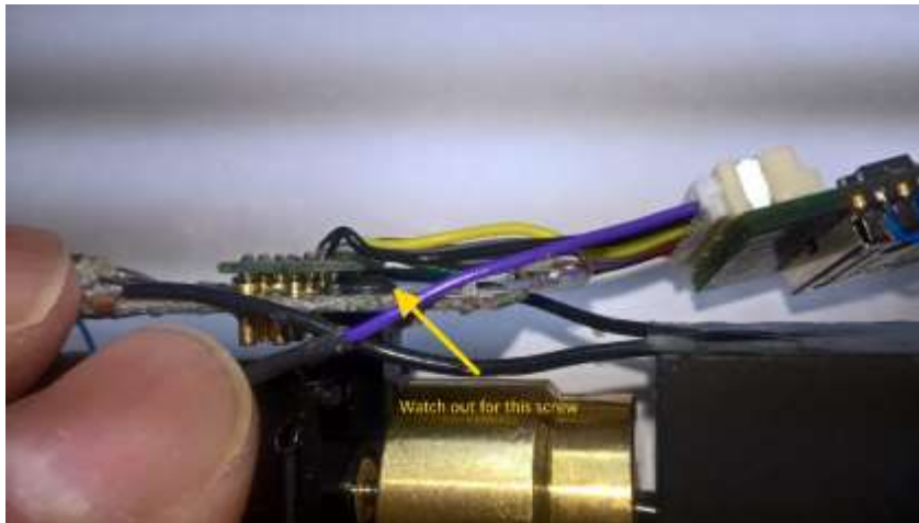
Figure 12 Make sure no wires touch the mounting screw.
