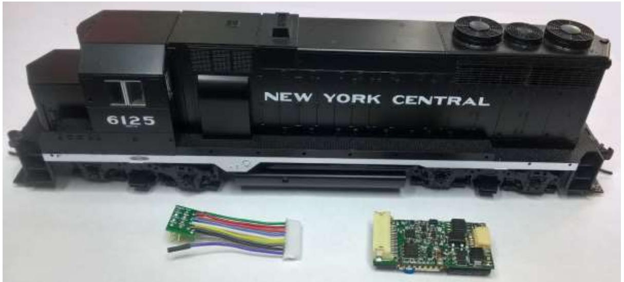
Figure 1 The Kato GP35 ph1a after removing the handrails with the WMH-20 Unit and selected 1.5" Standard Harness
