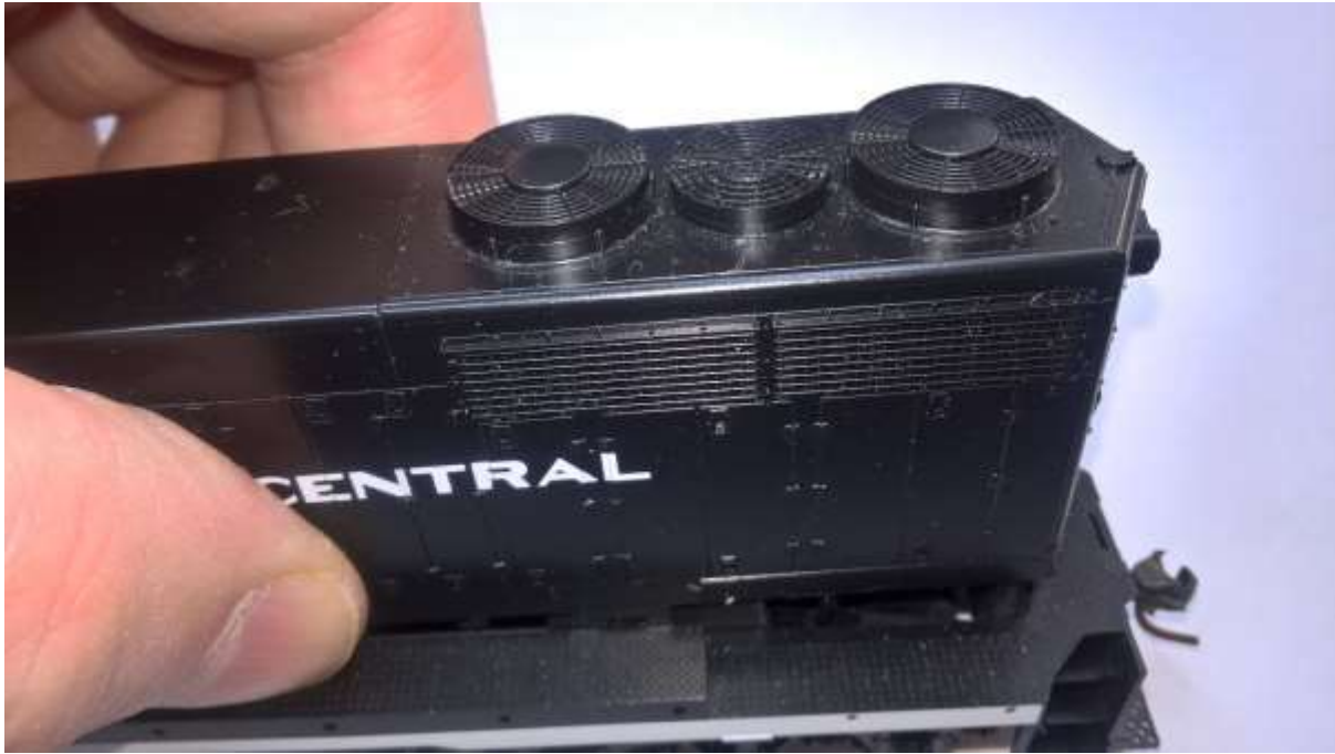
Figure 3 Lifting the body shell off the locomotive frame
