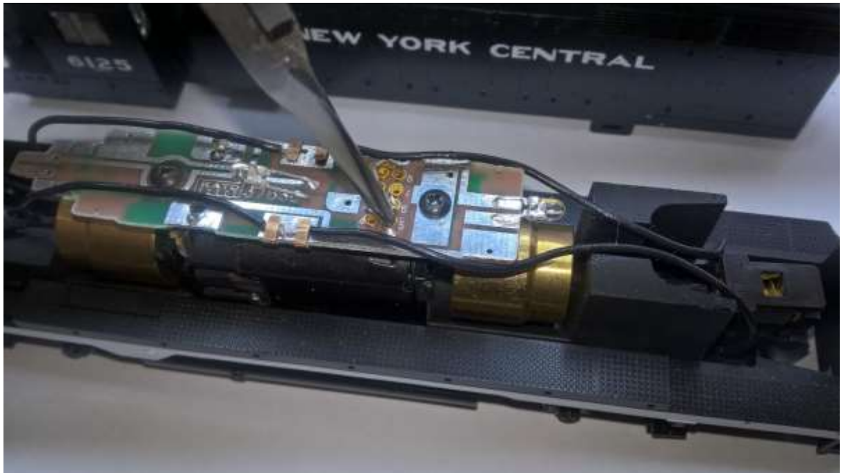
Figure 5 Removing the links from the 8-pin DCC socket
