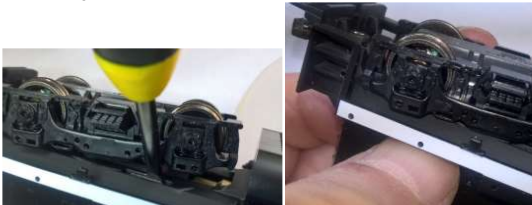
Figure 2 Releasing the plastic latches under the rear truck and easing the body off with the thumb nail
