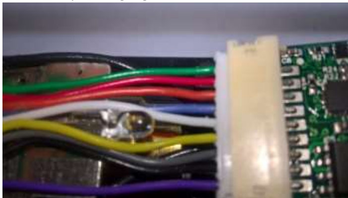
Figure 13 Tuck the colored leads down around the rear light LED.
