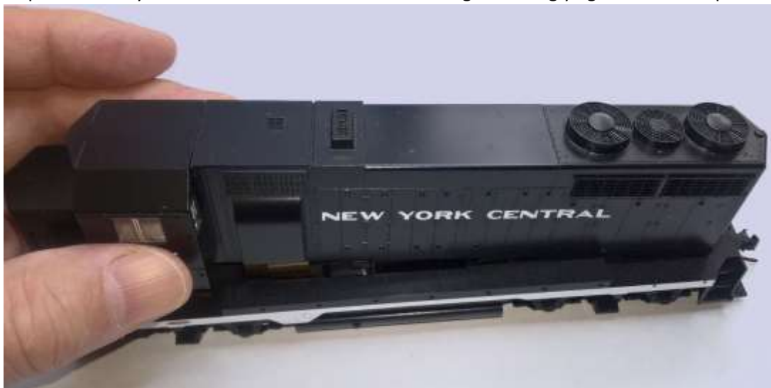
Figure 15 Complete the fitting of the body shell
